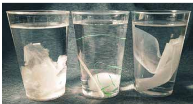
DAY 7 TEST. Common bathroom items after 7 days in water with minor agitation. From left: toilet tissue; Center: cotton ball, cotton swab, dental floss; Right: cleansing wipe. Only the septic safe toilet tissue is breaking down.
